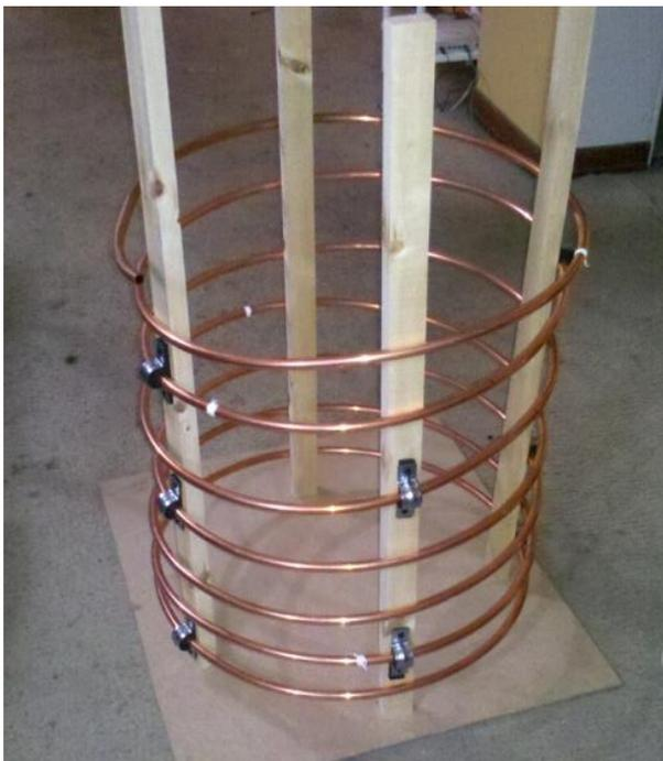
Figure 3. Source pipe of the reflectometer
