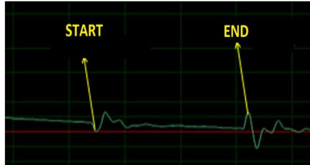
Figure 5. Reflections captured of a closed pipe
