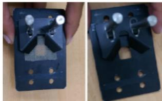
**Figure 3** VARIAN Cary5000 Spectrophotometer. Below: Holder with sample.
