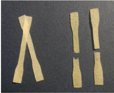
**Figure 2** Die cut covering samples, before and after mechanical tests.
