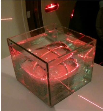
**Figure 1** Sample positioning in the tomograph and the linear accelerator.
