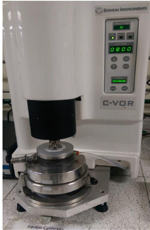
**Figure 4** Bohlin Instruments Rheometer, with sample submitted to tension by serrated parallel plates.
