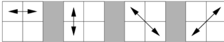
FIG. 1 Directions for calculation of Haralick texture features. From left to right: horizontal, vertical, transverse and diagonal.
