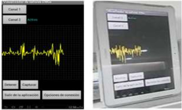
Figure 4 Display of the EMGs signals in the mobile device application
