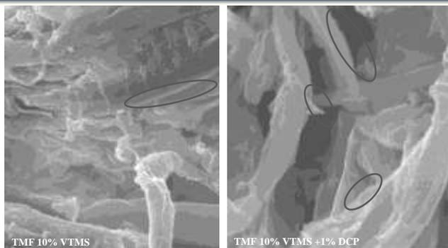
Figure 6 SEM 2000x. TMF coupled to VTMS/DCP
