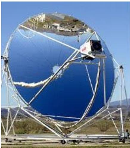
**Figure 2.** Parabolic dish type collector. [5]
