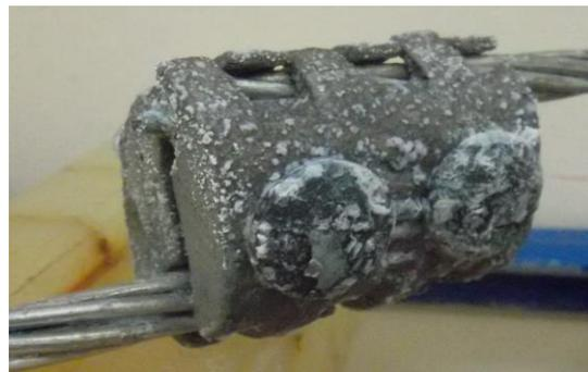
**Figure 2** Specimen after 337.5 h of exposure to the saline fog.
