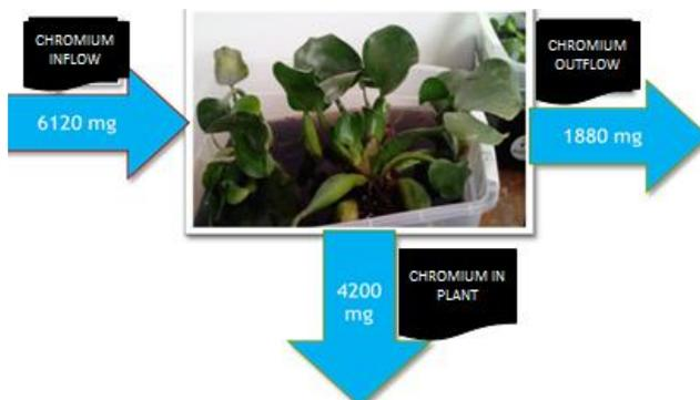
**Figure 8** Chromium Balance in experiment 2
