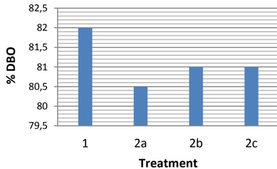
**Figure 5** BOD Removal (in %) in each of the treatments
